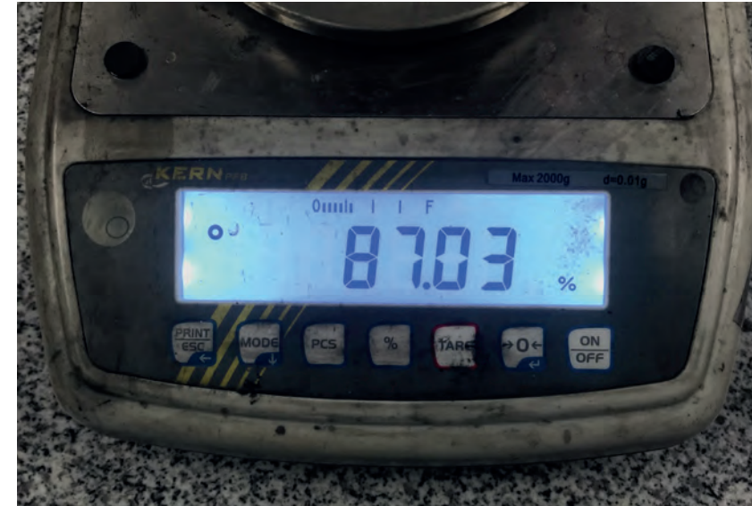
The lab scale shows the direct comparison: Approx. 15% weight reduction for a standard brake pad with an identical steel backing plate.
