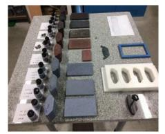
The above pictures show the production process starting with the drawing, the mold and the casted friction pads being glued to the backing plates. (The video showing the die-casting process can be seen at booth #30 at Eurobrake).
